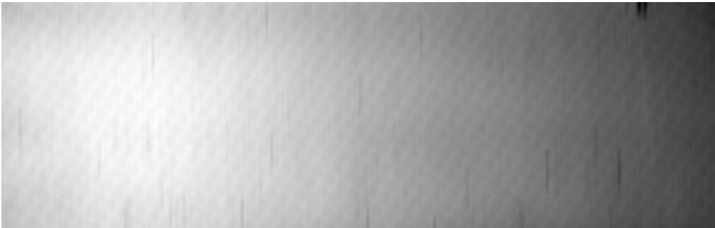
Figure 8: Beam image derived from the detector 1 flat field data. Since images were taken at several positions, the recovered beam image is wider than the detector.
