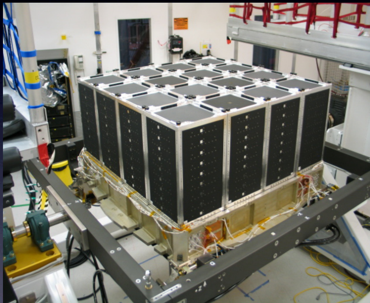
The LAT has 16 towers of particle detectors, seen here before the installation of the Anticoincidence Detector. Each tower contains a Tracker module and a Calorimeter module. The Data Acquisition System is located underneath the towers.
