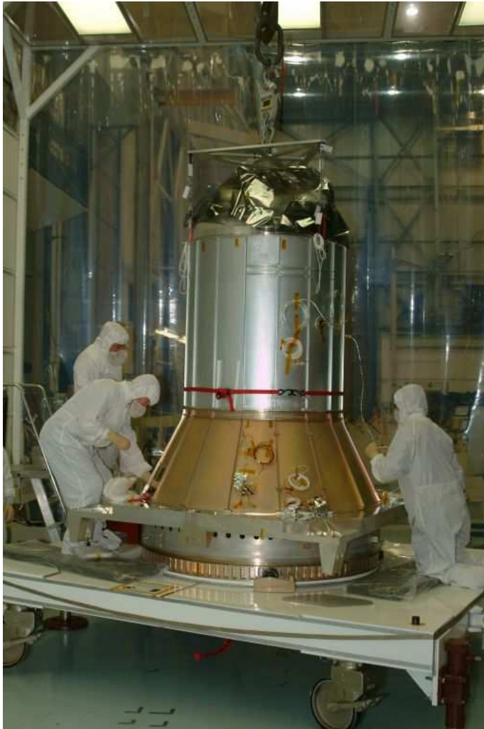
SDO's Propulsion Module being assembled in Building 10 (module was designed and built by GSFC)
