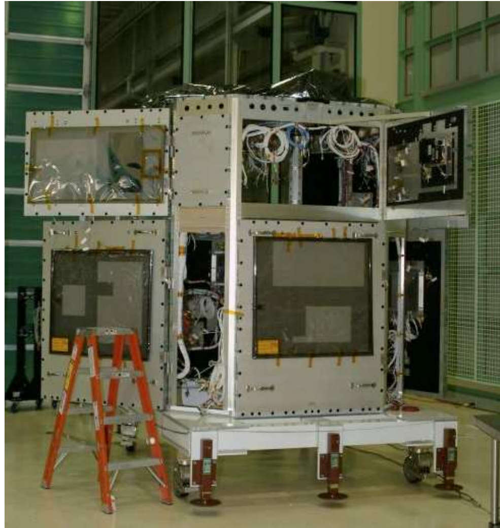
SDO's Flight Structure being assembled in the SCA in Building 7
