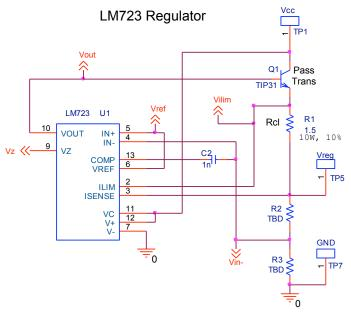
Use scope measure peak to peak voltage of ripples of V\_reg and V\_cc. Record enough settings to get a smooth curve of V\_bulk and V\_ripple versus output current. What would you estimate the minimum ripple rejection to be (in dB)? Is your estimate consistent with the specifications for 723?
