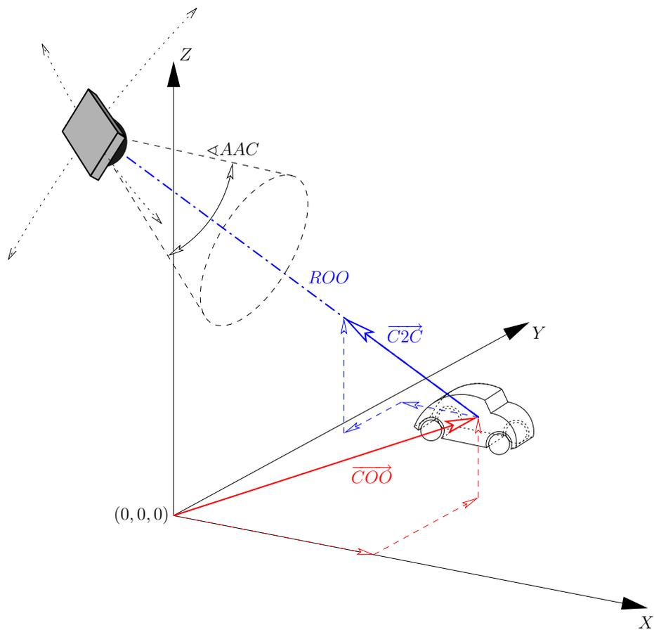
Figure 1: Camera and 3D object in the World System  $XYZ$ ; centre of orbit position vector  $\vec{COO}$ , centre of orbit to camera direction vector  $\vec{C2C}$ , radius of orbit  $ROO$ , aperture angle of camera  $\sphericalangle AAC$ .
