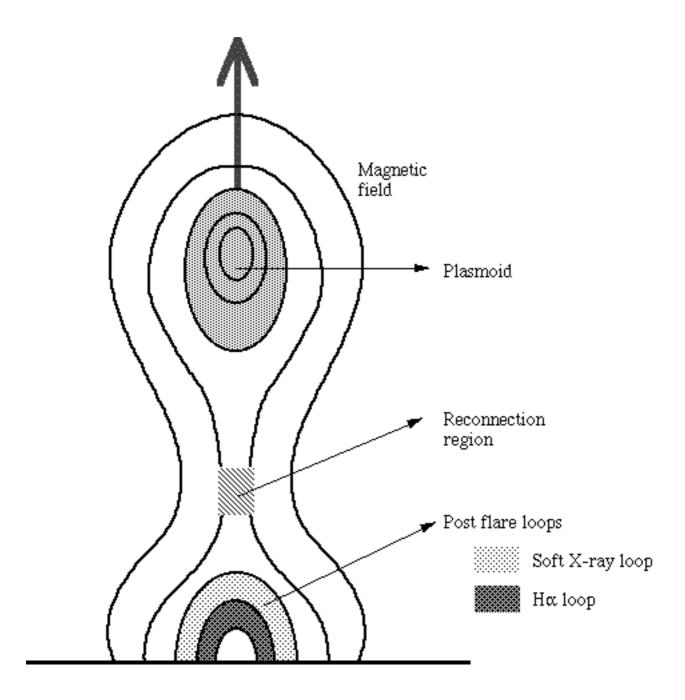
FIG. 1. 1.—Schematic illustration of eruptive flares. In the upper part, a magnetic island is formed and ejected upward as a plasma blob (plasmoid), while closed magnetic loops appear near the base, which can be observed as the postflare loops.
