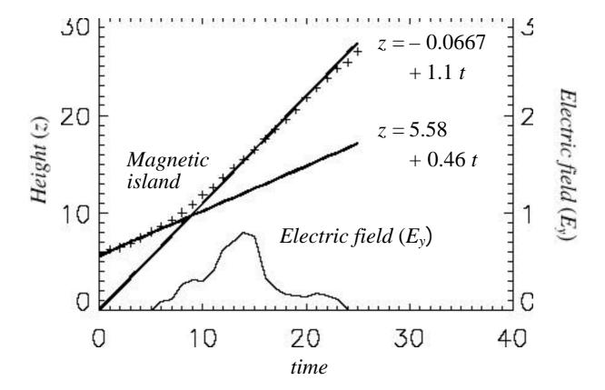
FIG. 3. 3.—Time variations of the *y*-component of the electric field ( $E_y$ ) at a neutral point and the height of a magnetic island of model r3, each of which are represented by a thin solid line and crosses (+), respectively. Two thick solid lines represent the result of the line-fittings applied to the time variation of the height of the magnetic island. The time ranges of such line-fittings are 0 t 5 for the first one and 15 t 17 for the second one.
