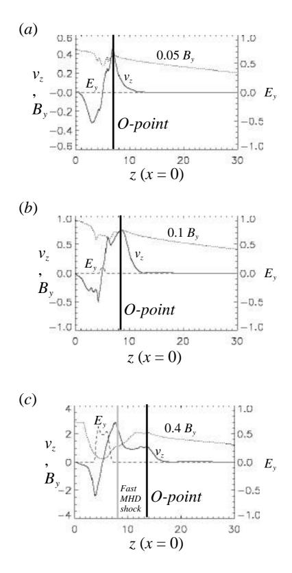
FIG. 3. 4a–4c.–Spacial distributions along the *z*-axis of the perpendicular magnetic field ( $B_y$ , dotted line), vertical velocity ( $v_z$ , solid line), and neutral-point electric field ( $E_y$ , broken line): (a) at t = 3, (b) at t = 6, and (c) at t = 12. The position of an O-point is also represented by a vertical thick solid line, while the position of a fast MHD shock is shown by a vertical thick broken line.
