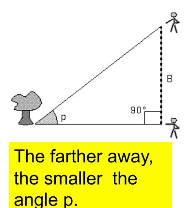
The distance **d** is determined by the **baseline length B** and angle **p** (**parallax**) as:
