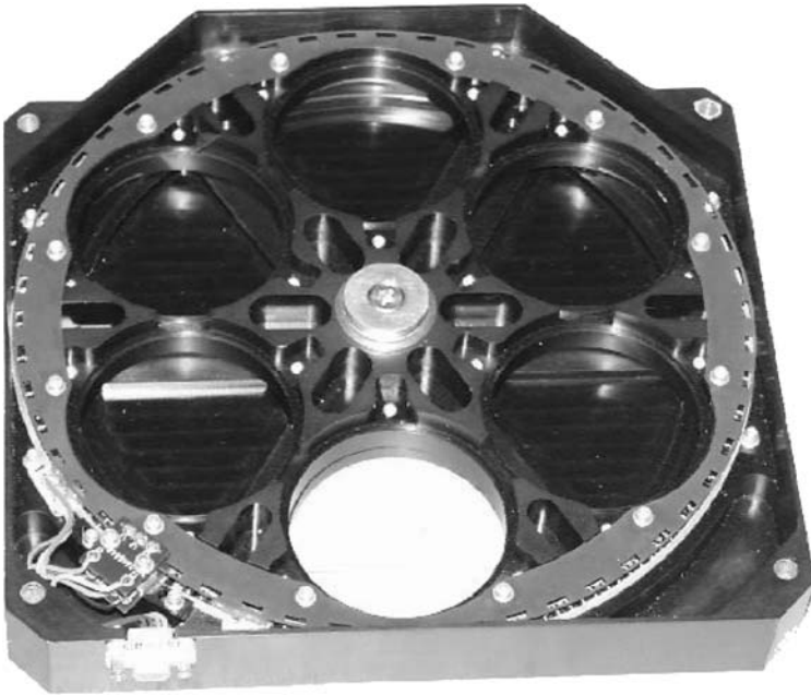
Figure 6 One of the two XRT filter wheels, each of which holds five filters and has one open position.
