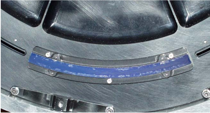
Figure 5 One of the six annular aluminized polyimide entrance filters of the XRT.
