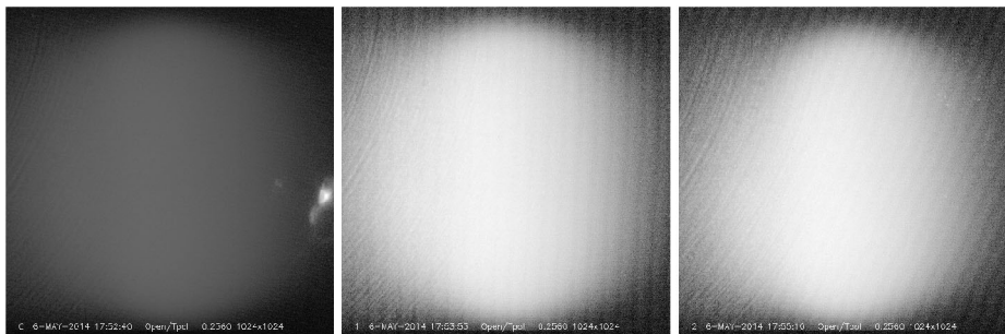
Figure 8 Three consecutive images obtained with the Ti-poly filter during the 6 May 2014 measurement. Pixels with higher intensity are shown brighter here to highlight the faint structures. Left: obtained at 17:52:40 UT. Center: obtained at 17:53:55 UT. Right: obtained at 17:55:10 UT. The center image has the stray-light pattern that is suitable for correction.
