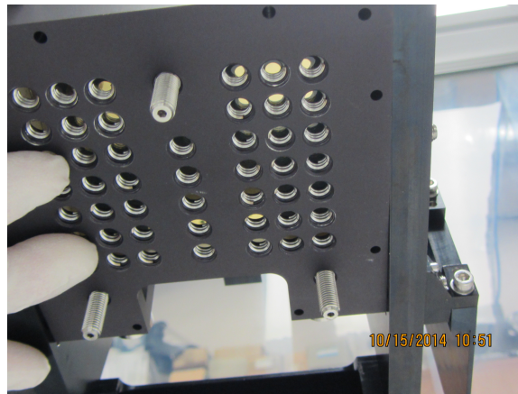
Figure 2.3: Back plate of the primary mirror mount. The three threaded shafts are the vlier screws that push the primary against the tip/tilt/focus constraints. The grid of threaded holes accepts vlier screws to apply controlled forces to the back of the mirror in an effort to correct the distorted figure.
