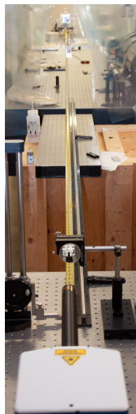
Figure 6.1: Test setup for measuring primary mirror radius of curvature.
