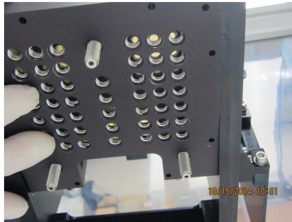
Figure 6.3: Back plate of the primary mirror mount. The three threaded shafts are the vlier screws that push the primary against the tip/tilt/focus constraints. The grid of threaded holes accepts vlier screws to apply controlled forces to the back of the mirror in an effort to correct the distorted figure.
