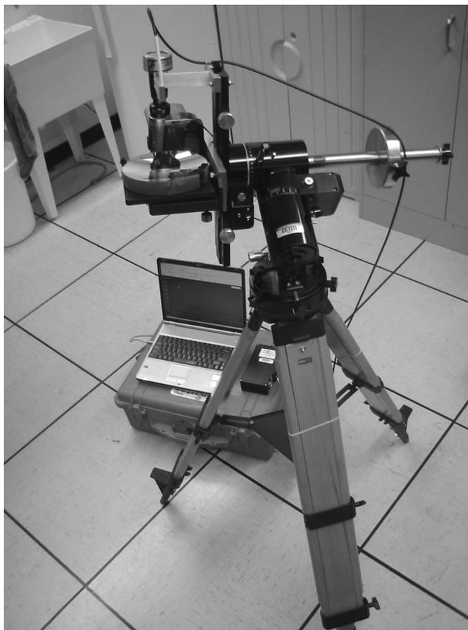
Fig. 1.— A picture of the instrument setup as reconstructed in the lab for one of the many post-eclipse tests. The spectrograph can be seen sitting next to the computer. The black fiber optic cable connects from prime focus to the spectrograph. The video camera is co-mounted with the telescope and shown with its solar filter on.
